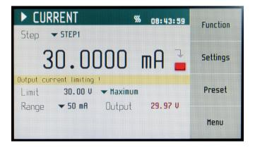
Press the STEP button to start the ramp function.
