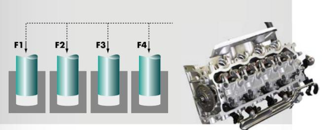
Multichannel monitoring of joining process in cylinder head assembly. The synchronous process during the assembly of valve seating rings and valve guides is measured and analyzed. DigiControl PC software logs and visualizes the process data from up to 32 controllers.
