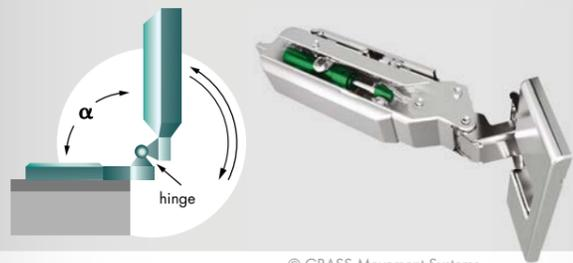
Measuring the correct torque/angle response in final testing of hinges.
