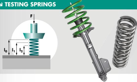
Testing of spring constant and hysteresis between applying and removing load.
