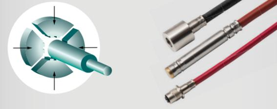
To monitor crimping processes, the force applied by the jaw segments to the material deformation is analyzed as a force/time curve. Wear to a jaw segment or breakage can be detected.
