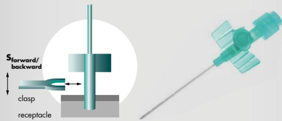
Testing the ease of movement of a venous canula over the length of the steel insertion needle. The clasp holds the canula and moves it up and back over the needle.
