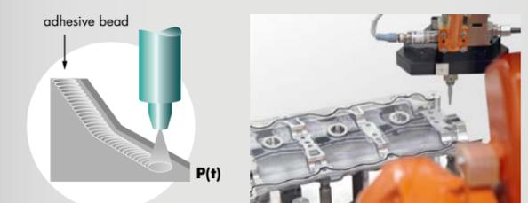
Checking for continuous application of adhesive beads, e.g. to prevent leaks from gaps in the adhesive joint. This is done by monitoring the pressure/time curve in the dispensing line.
