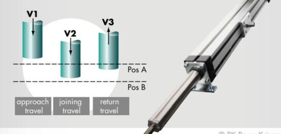
When monitoring the joining process on servo-electric joining axes, the relevant process variables can be measured either directly at the front end of the joining axis or indirectly, e.g. from the motor rotation.
