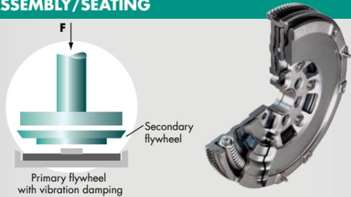
Monitoring primary and secondary flywheels of a dual mass flywheel during assembly.
