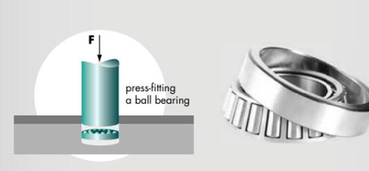
Monitoring the press-insertion of ball bearings in bearing cups.
