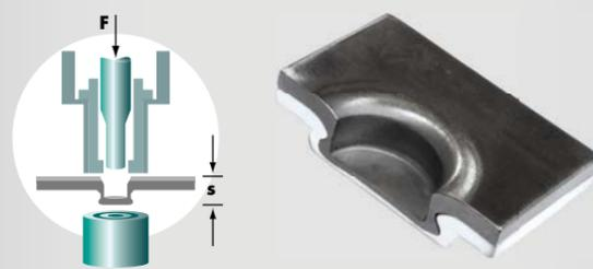
The flow process produced in the two sheet metal parts by the clinching stamp and die is monitored by a force/displacement measurement.
