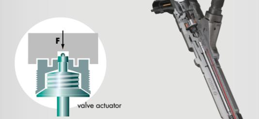
Press-insertion and precise positioning of the valve actuating elements are monitored during assembly of common-rail injectors.
