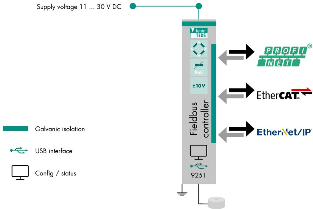
Block diagram – multichannel application with universal instrumentation amplifier, fieldbus controller with measuring input and load cells
